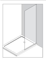
Using two people fit the fixed panel into the channels ensuring it is pushed in firmly into the wall channel.
