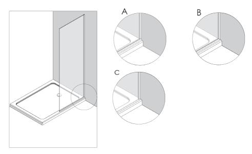
The channels supplied allow varying options for fitting:
