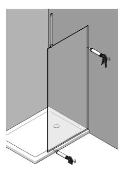
Apply silicone sealant to the outside of the fame where the channels meet the tiles and tray.
