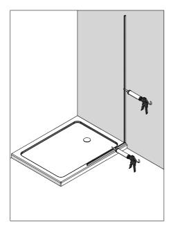
Apply glazing silicone sealant to the interior of the channels
