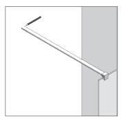
Mark the wall or ceiling to indicate the location for the wall clamp.
