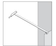
Or loosely fit the clamp to the screen and cut the wall bar to the required length using a hacksaw.
