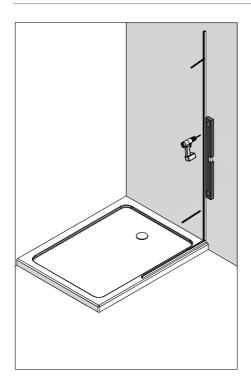
Mark the wall and channel for drilling avoiding areas such as tile edges.
