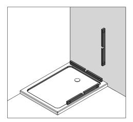
Prior to install check the tray is flat and square to the wall.
