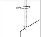
Depending where you have wall bar or ceiling bar: loosely fit the clamp to the screen and cut the ceiling bar to the required length using a hacksaw.
