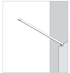
Fully secure the wall or ceiling bar by tightening the grub screws.
